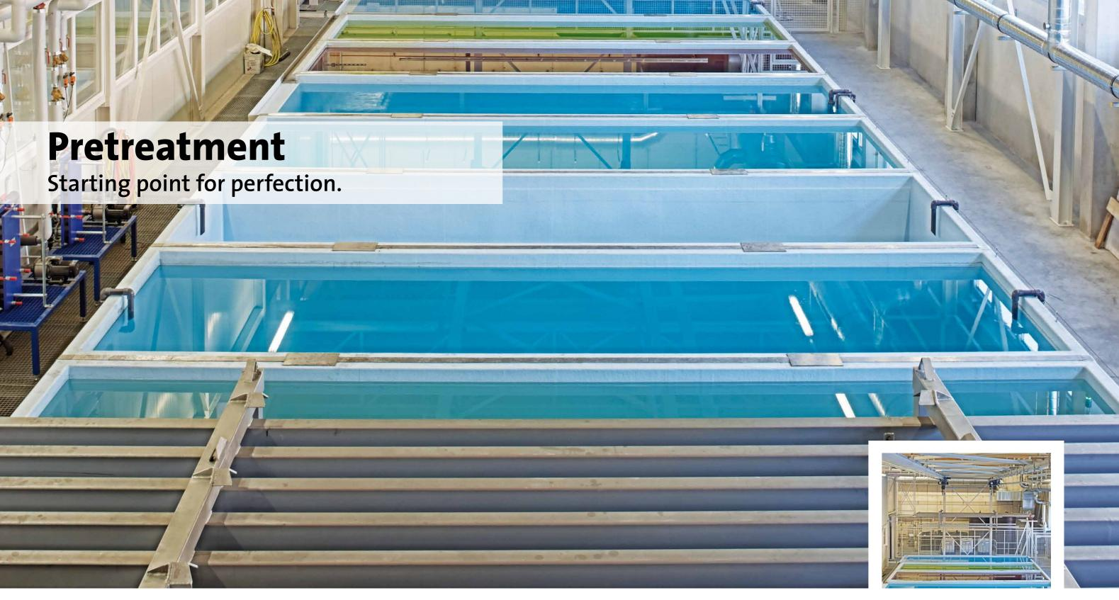
Perfection and quality can only be ensured by properly treated raw materials. Paint and powder adhere better to specifically pretreated parts, while corrosion protection is increased. Therefore contaminations are thoroughly removed from the surfaces using special procedures. The choice of suitable pretreatment methods is thus a deciding factor in systems engineering
