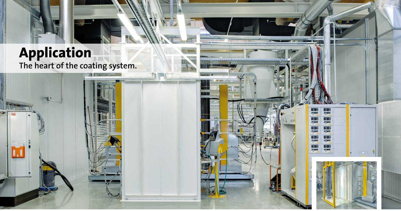
With the powder application the parts are treated with electrostatically charged powder paints. This work process serves as much for the refinement as for the protection of the surface. According to the respective requirement profile of the system, the suitable application system will be selected, designed and produced.
